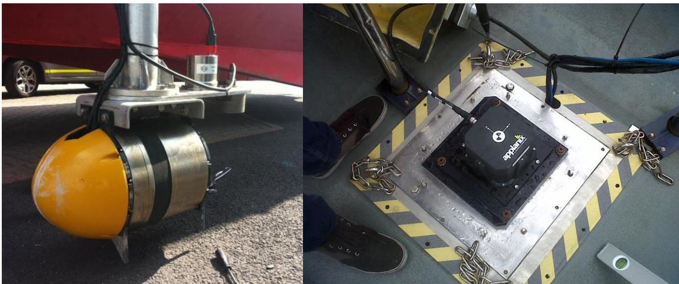
Figure 2: Left: Transducer (installed on CSV Thames Guardian). Right: Installed Inertial Measurement Unit (IMU)
